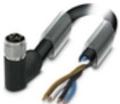
Power cable, 4-position, PUR halogen-free, black-gray RAL 7021, free cable end, on Socket angled M12, coding: T, cable length: 10 m, For direct current up to 12 A/63 V
