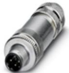
Data connector, Ethernet/PROFINET CAT5 (100 Mbps), 4-position, shielded, Plug straight M12, Coding: D, Screw connection, knurl material: Zinc die-cast, nickel-plated, cable gland Pg9, external cable diameter 6 mm ... 8 mm
