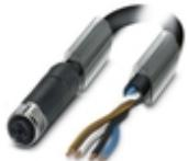
Power cable, 4-position, PUR halogen-free, black-gray RAL 7021, free cable end, on Socket straight M12, coding: T, cable length: 2 m, For direct current up to 12 A/63 V
