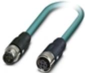
Network cable, Ethernet CAT5 (100 Mbps), 4-position, shielded, Plug straight M12 SPEEDCON / IP67, coding: D, on Socket straight M12 SPEEDCON / IP67, coding: D, cable length: Free input (0.2 ... 40.0 m)
