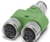
Y distributor, 4-position, Plug straight M12 SPEEDCON, coding: A, on Socket straight M12 SPEEDCON, coding: A, PIN 2+4 bridged and Socket straight M12 SPEEDCON, coding: A, PIN 2+4 bridged, Thread M12 socket not rotatable
