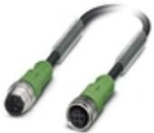
Sensor/actuator cable, 3-position, Variable cable type, Plug straight M12, coding: A, on Socket straight M12, coding: A, cable length: Free input (0.2 ... 40.0 m)
