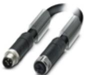
Power cable, 4-position, PUR halogen-free, black-gray RAL 7021, Plug straight M12, coding: T, on Socket straight M12, coding: T, cable length: 5 m, For direct current up to 12 A/63 V
