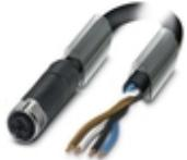
Power cable, 4-position, PUR halogen-free, black-gray RAL 7021, free cable end, on Socket straight M12, coding: T, cable length: 1 m, For direct current up to 12 A/63 V
