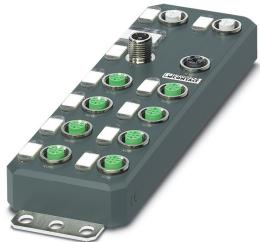
Axioline E, Digital input device, EtherNet/IP™, M12 fast connection technology, Digital inputs: 16, 24 V DC, connection method: 4-conductor, Plastic housing, degree of protection: IP65/IP67
