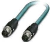
Network cable, Ethernet CAT5 (100 Mbps), 4-position, shielded, Plug straight M12 SPEEDCON / IP67, coding: D, on Plug straight M12 SPEEDCON / IP67, coding: D, cable length: Free input (0.2 ... 40.0 m)
