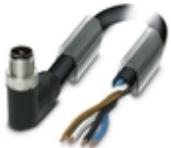
Power cable, 4-position, PUR halogen-free, black-gray RAL 7021, Plug angled M12, coding: T, on free cable end, cable length: 10 m, For direct current up to 12 A/63 V
