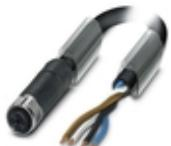
Power cable, 4-position, PUR halogen-free, black-gray RAL 7021, free cable end, on Socket straight M12, coding: T, cable length: 10 m, For direct current up to 12 A/63 V
