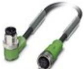
Sensor/actuator cable, 4-position, Variable cable type, Plug angled M12, coding: A, on Socket straight M12, coding: A, cable length: Free input (0.2 ... 40.0 m)
