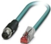
Network cable, Ethernet CAT5 (100 Mbps), 4-position, Variable cable type, shielded, Plug straight M12 SPEEDCON / IP67, coding: D, on Plug straight RJ45 / IP20, cable length: Free input (0.2 ... 40.0 m)
