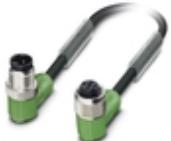
Sensor/actuator cable, 4-position, Variable cable type, Plug angled M12, coding: A, on Socket angled M12, coding: A, cable length: Free input (0.2 ... 40.0 m)
