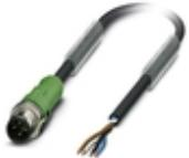
Sensor/actuator cable, 4-position, Variable cable type, Plug straight M12 SPEEDCON, coding: A, on free cable end, cable length: Free input (0.2 ... 40.0 m)
