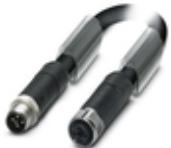
Power cable, 4-position, PUR halogen-free, black-gray RAL 7021, Plug straight M12, coding: T, on Socket straight M12, coding: T, cable length: 0.3 m, For direct current up to 12 A/63 V
