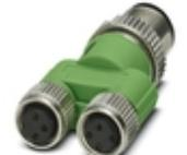
Y distributor, 4-position, Plug straight M12 SPEEDCON, coding: A, on Socket straight M8, coding: A and Socket straight M8, coding: A
